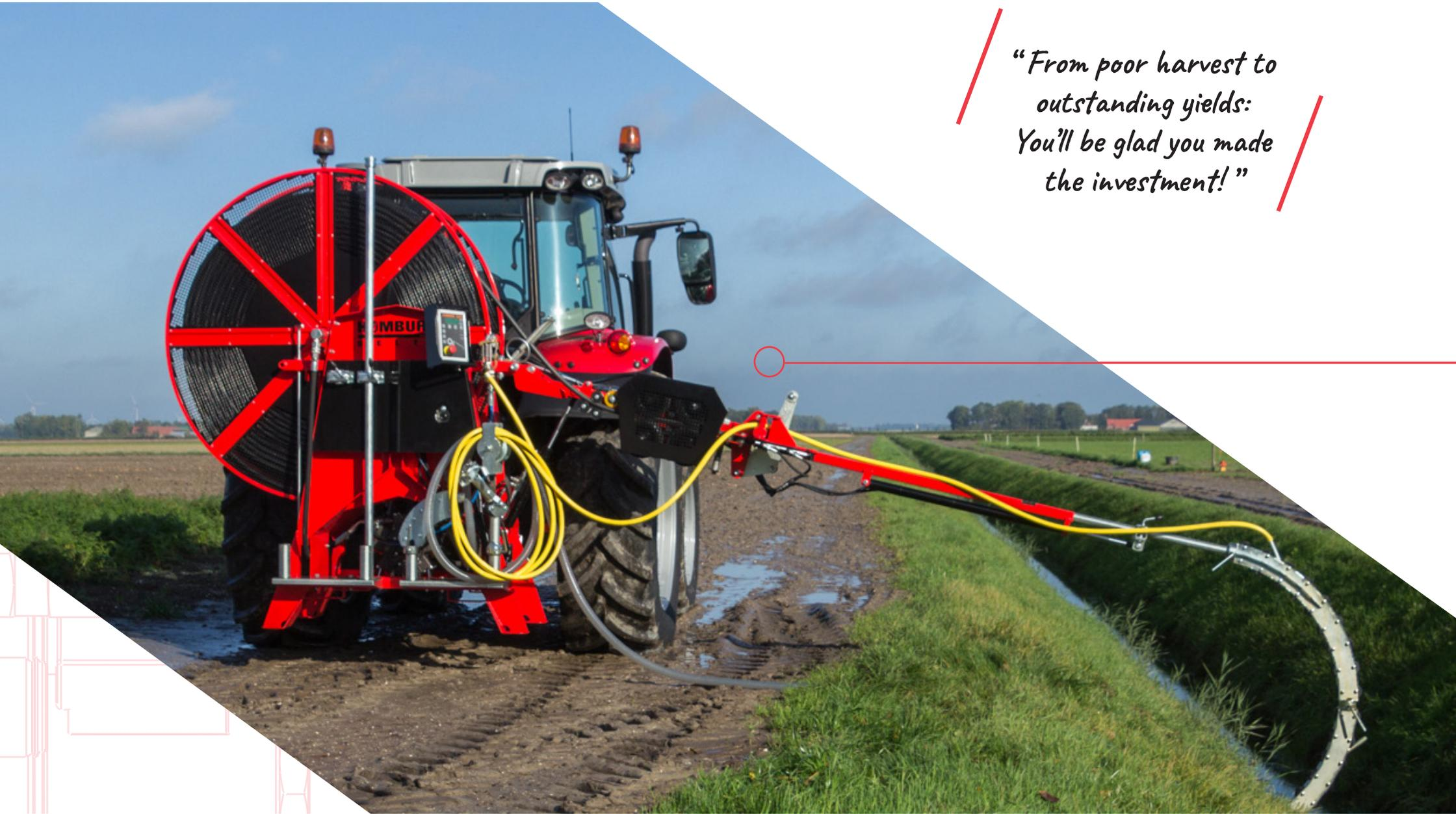
The DELTA offers more ease of use as a draincleaner than the JUNIOR. This is the ideal machine for anyone who maintains drainage systems on a frequent basis and needs to cover a large area. This is because it offers hydraulically operated height adjustment, extension, retraction and folding of the drainage arm and length adjustment of the guide arm.
